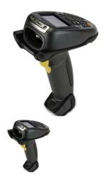
Combines advanced 1D/2D barcode, DPM and image capture with the ability to key in and view data - plus 802.11a/b/g and Bluetooth connectivity options.
