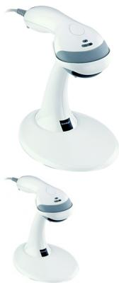
Voyager and VoyagerCG hand-held, single-line laser scanners feature patented automatic infrared activation and decode all standard 1D bar codes, including GS1 DataBar™. VoyagerCG also includes CodeGate® technology for menu scanning applications. CodeGate zeroes in on the desired code and completes data transmission with the push of a single button.
